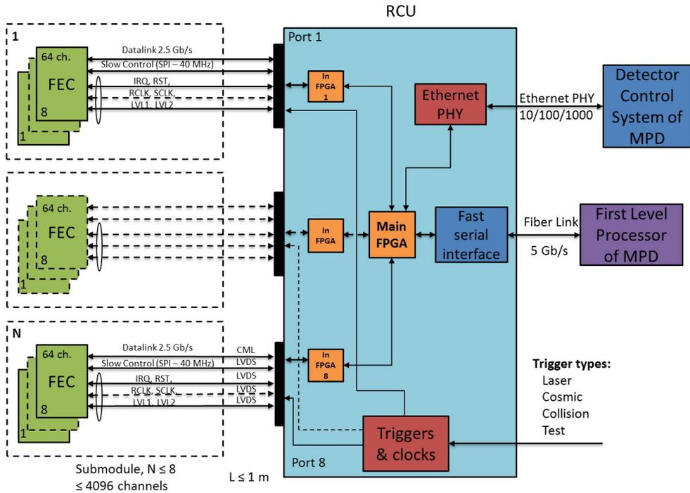
Figure 1: Structural scheme of one chamber readout
