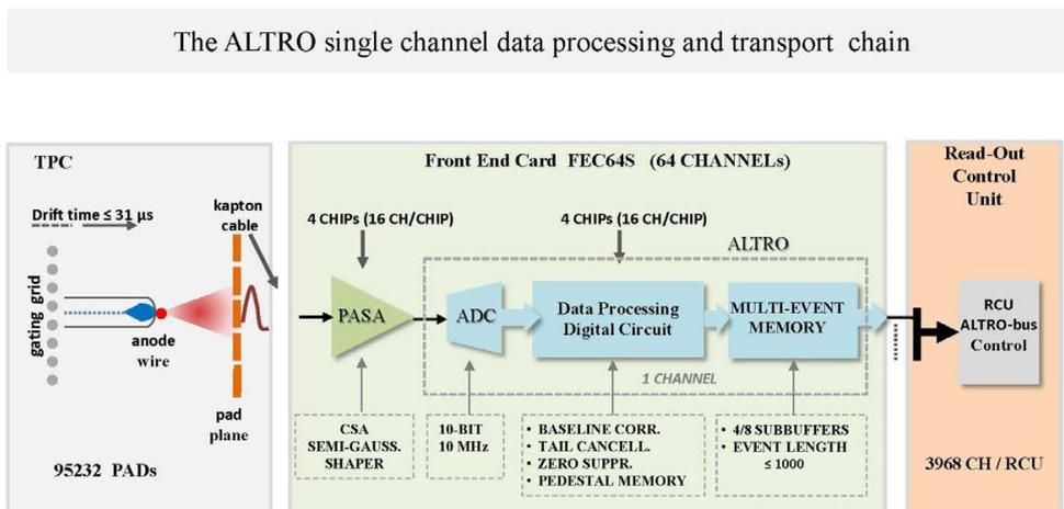
Figure 6: Single channel structural scheme
