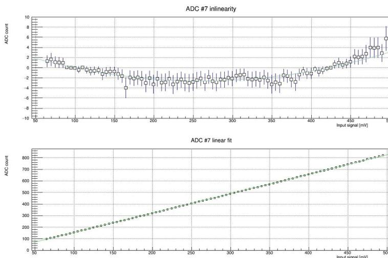
Figure 8: FEC linearity. Top graph shows the difference between the measured value and the linear fit. The bottom graph demonstrates FEC response to the input signal
