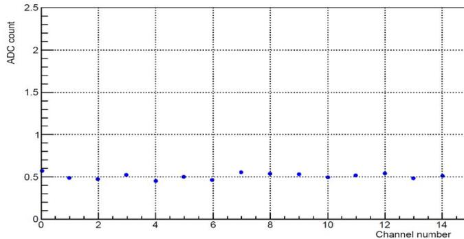
Figure 7: Noise value at 16 FECs channels (without cable)
