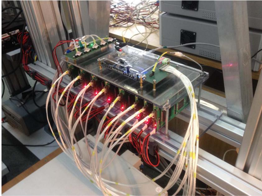
Figure 9: Test system for eight cards. 1) FECs array (512 ch. in total), 2) clocks and control signal distribution card, 3) RCU emulator
