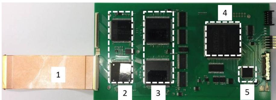
Figure 4: Front-End Card FEC64S. 1) Cable between the detector and FEC; 2) PASA chips - low noise amplification of the signal; 3) ALTRO chips - digitization and processing; 4) FPGA board controller; 5) Serializer/Deserializer chip
