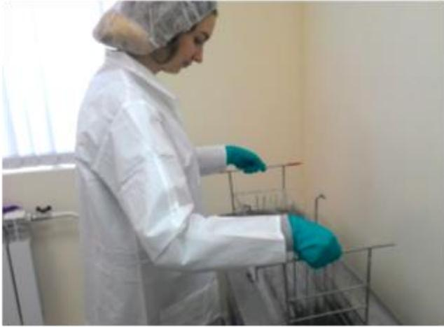
**Figure 3.36:** Ultrasonic cleaning of glass.
