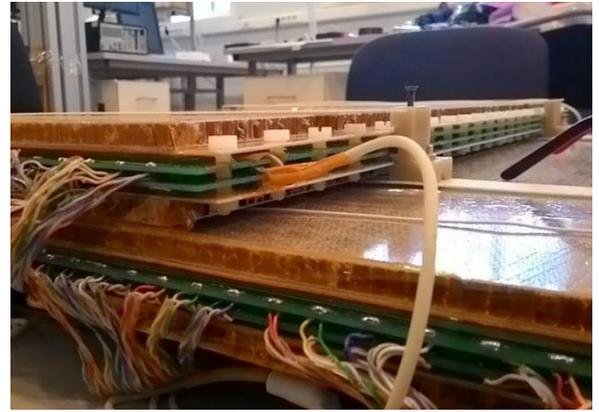
**Figure 2.4:** Readout from three stacks of the MRPC.
