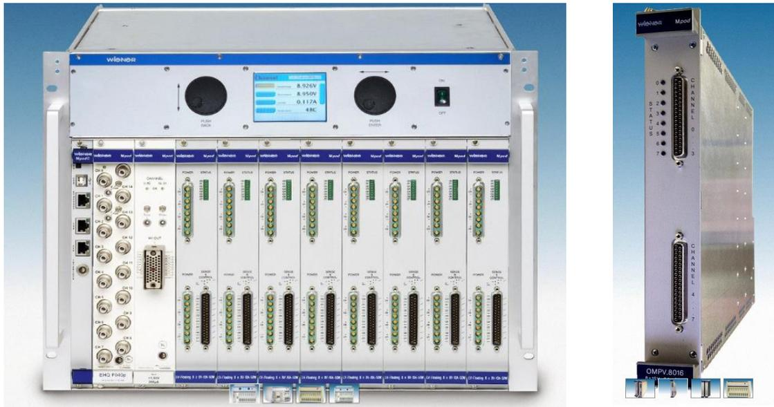
**Figure. 4.8:** "W-IE-NE-R" MPod crate and 8-channel LV power supply MPV 8016I.
