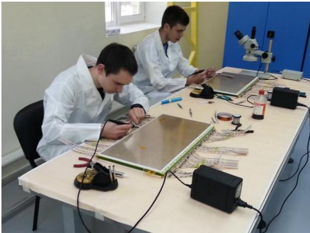
**Figure 3.40:** Soldering of the signal cables.
