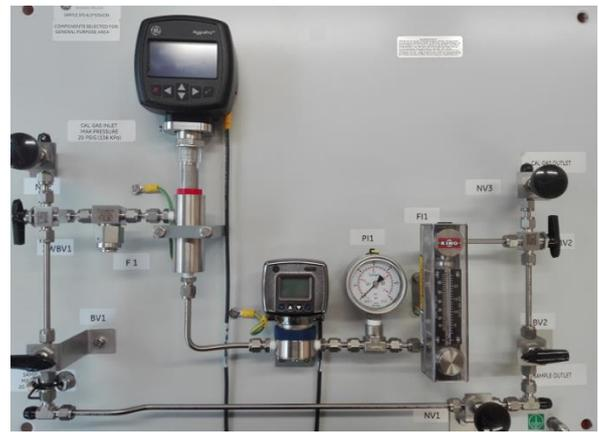
**Figure 4.4:** Scheme and photo of the gas analyzing system.
