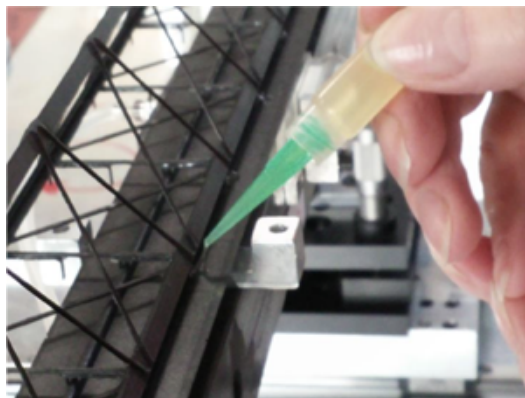
Figure 3.30: Space Frame gluing to the Cold Plate.
