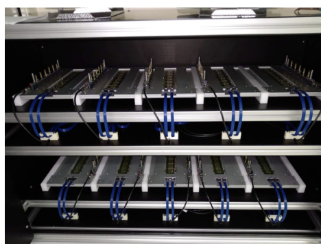
Figure 3.24: Endurance test box holding 10 HICs inside their carrier plates.
