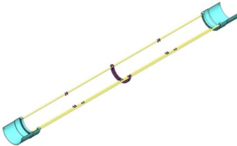
Figure 3.38: Possible design of the Inner Barrel chassis
