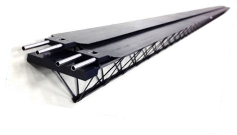
Figure 4.2: One of 42 OB MPD ITS staves cooling sections.
