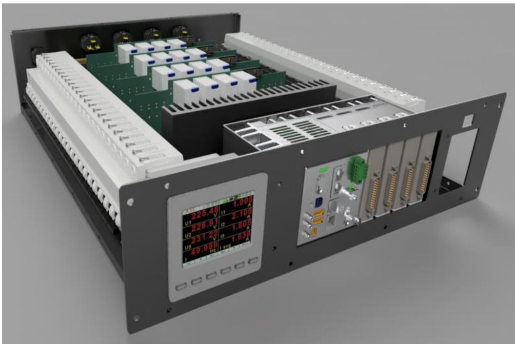
Figure 9—27; Visualization of the IPD without cover housing – Front View.
