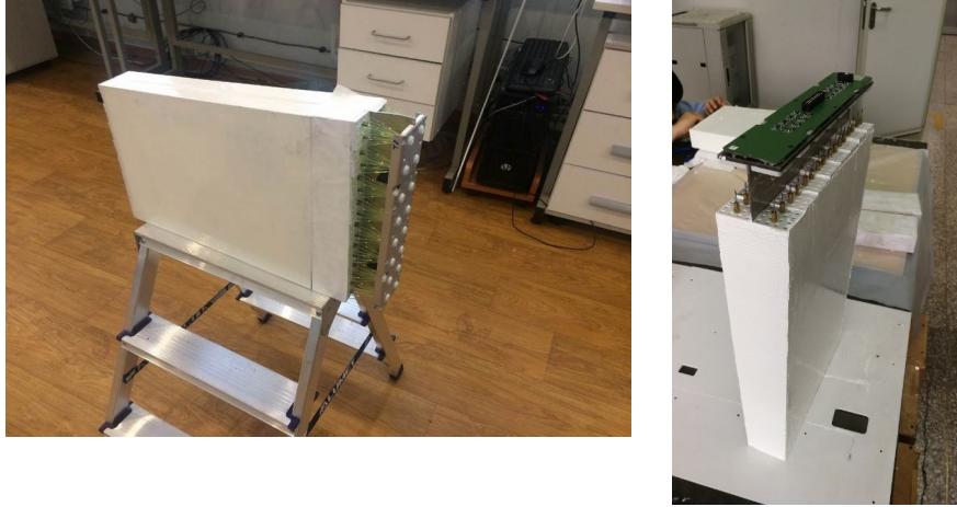
Figure 3.1.4: The module prototypes made for the MPD in Institute for High Energy Physics (Protvino) and in Tsinghua University (Beijing, China) are shown in the left and the right panels, correspondingly.
