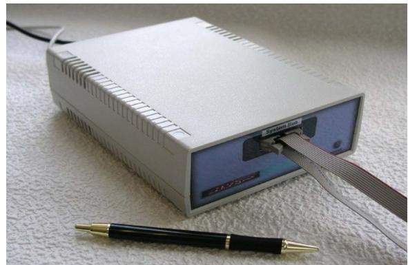
Figure 3.3.1.2: Control Units (Communication base voltage generation).
